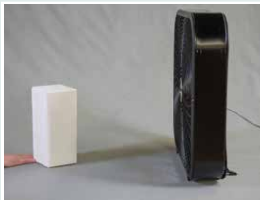
Figure 8: Place building angled in front of fan
